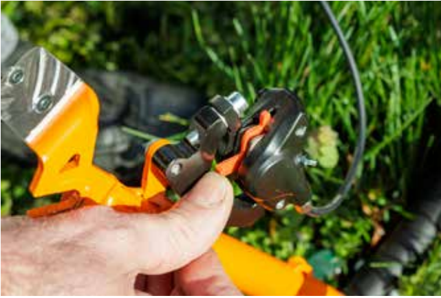
6. Remove the plastic wedge positioned between the pads.
