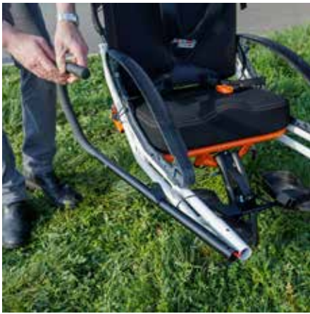
13. Unfold the arms and snap the two parts together.
