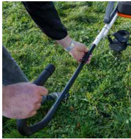
13. Unfold the arms and snap the two parts together.
